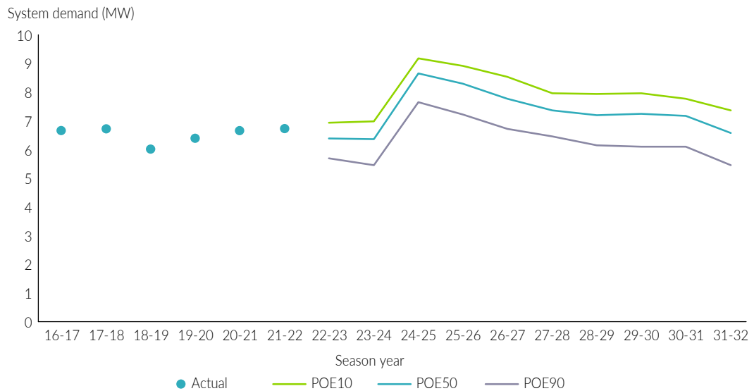
Figure 10: Historical and forecast minimum system demand in the Katherine node by season year (year ending 31 August), 2016-17 to 2031-32
