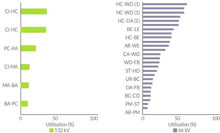
The planned upgrades between Hudson Creek and Palmerston appear to be effective in reducing flows on the existing circuits in that corridor. Entura notes the ongoing load balancing issues required in the Weddell 66 kV loop. The Archer-Palmerston 66 kV line will reduce the reliance on generation from Weddell power station to manage network flows.
