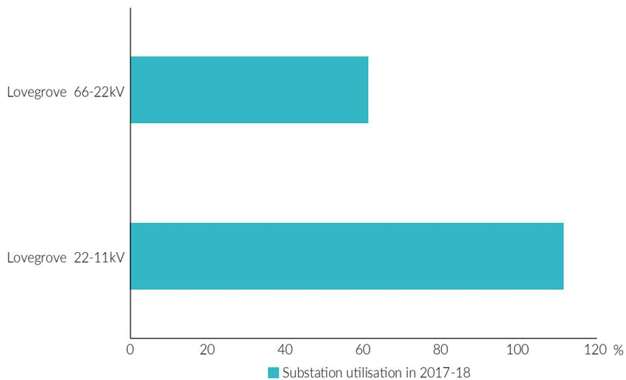
Entura's analysis shows the load on the Lovegrove 22:11 kV transformers exceeds the contingency cyclic rating. This differs from PWC's analysis, which shows it is just sufficient to supply the POE 10 demand. Entura takes a more conservative approach to the assessment of N-1 than PWC. PWC plans to upgrade these transformers in 2020-21.
