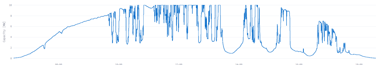
Figure 4 – Typical generation profile of a major grid connected solar PV generator demonstrating output volatility 9
