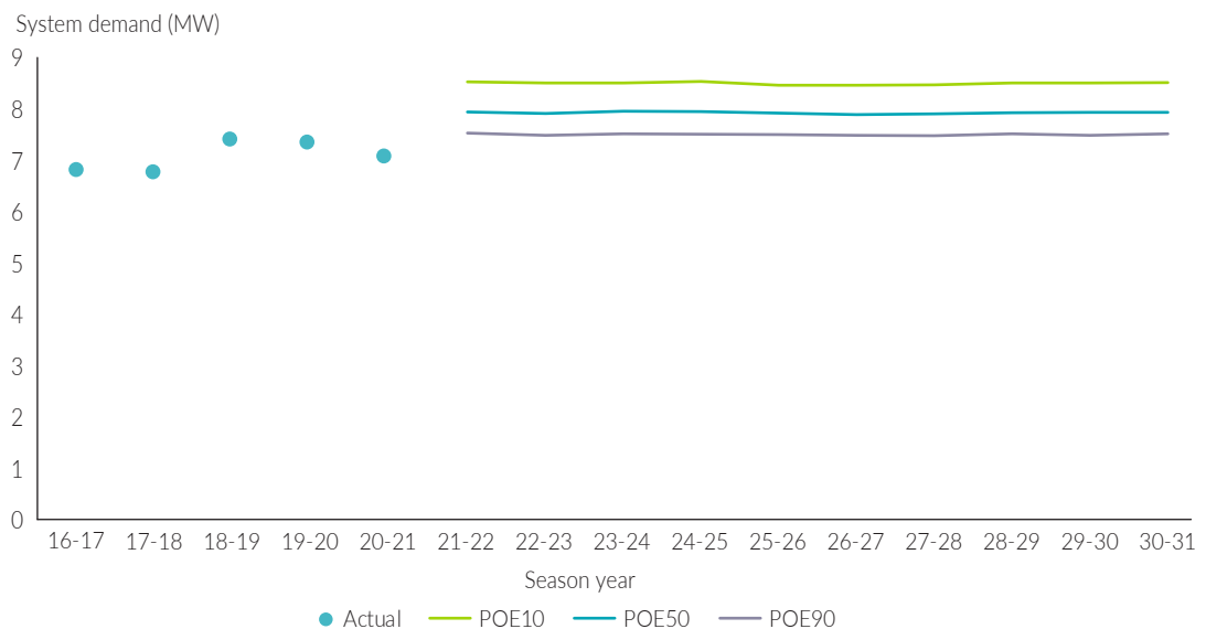
Figure 26: Historical and forecast maximum system demand for Tennant Creek by season year (year ending 31 August), 2016-17 to 2030-31
